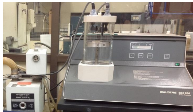
Figure 7.2: Vacuum chamber from carbon sputtering machine CED-30
