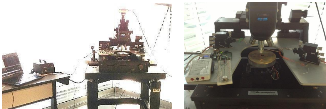
Figure 6.8: Experimental setup: complete (left), micromanipulator station plus DAQ and signal conditioning (right)
