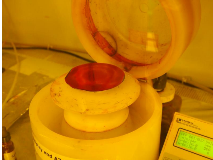
Figure 2.3: Resist Spinner with wafer covered in photoresist
